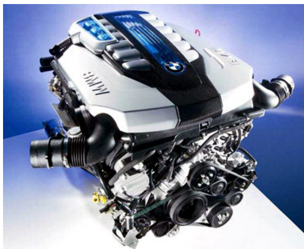
Hydrogen internal combustion engines are a relatively mature and inexpensive technology. The above image shows BMW's 6L V12 engine which can run on hydrogen or petrol. Photo: BMW
