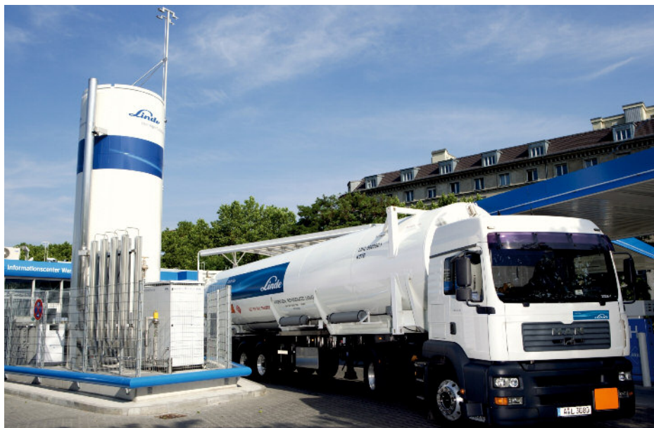
Liquid hydrogen storage is commonly used to transport hydrogen over long distances. Photo: Linde.
