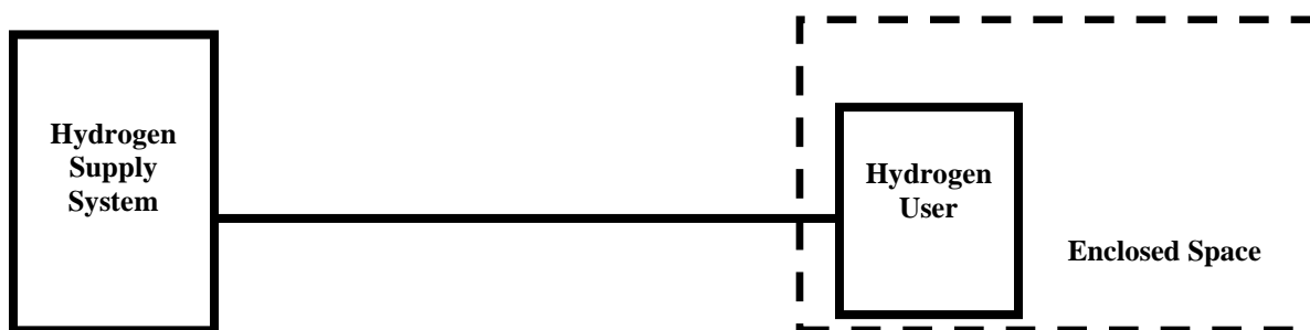
Figure B.1. Outdoor hydrogen supply system for indoor use
